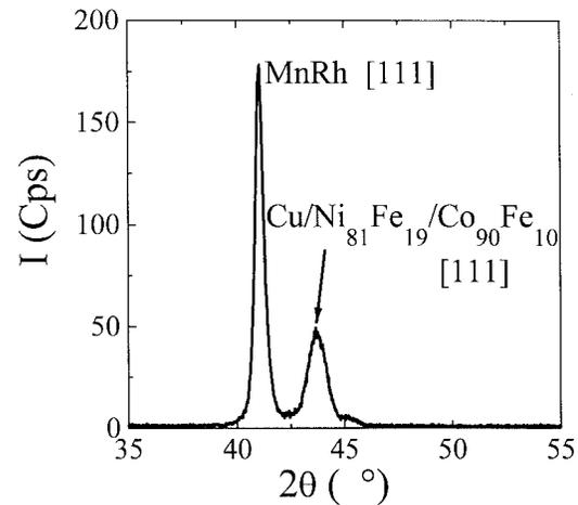
Fig. 1. X-ray spectra for the spin valve coupon sample Si/Ta ( $50 \text{ \AA}$ )/ $\text{Ni}_{81}\text{Fe}_{19}$  ( $60 \text{ \AA}$ )/ $\text{Co}_{90}\text{Fe}_{10}$  ( $5 \text{ \AA}$ )/Cu ( $23 \text{ \AA}$ )/ $\text{Co}_{90}\text{Fe}_{10}$  ( $22 \text{ \AA}$ )/ $\text{Mn}_{78}\text{Rh}_{22}$  ( $170 \text{ \AA}$ )/Ta ( $50 \text{ \AA}$ ).  $\text{Mn}_{78}\text{Rh}_{22}$  and  $\text{Cu/Ni}_{81}\text{Fe}_{19}/\text{Co}_{90}\text{Fe}_{10}$  peaks are observed.
