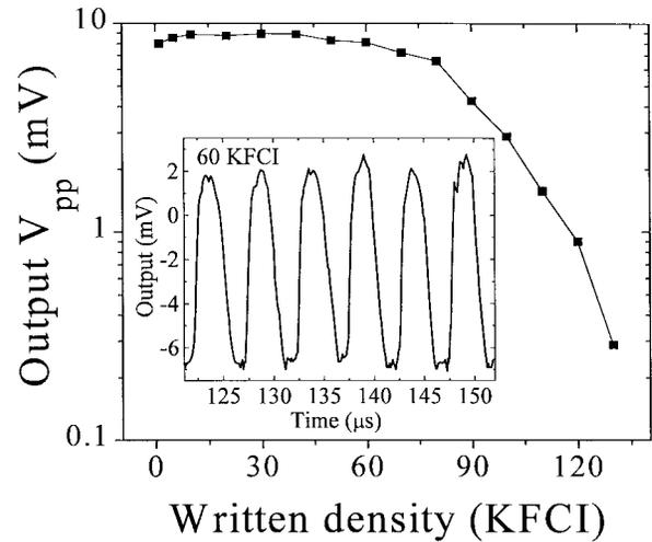
Fig. 7. Roll-off curve for the fundamental component of a  $5 \times 1 \mu\text{m}^2$   $\text{Mn}_{78}\text{Rh}_{22}$ -biased spin valve tape head measured on a 1850 Oe metal particle tape. The inset shows the output voltage at 60 kfcI.
