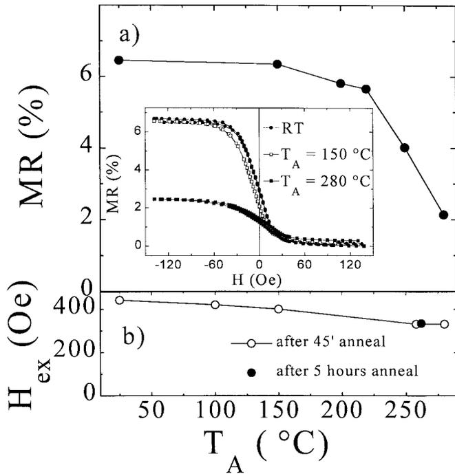
Fig. 6. (a) MR signal of the  $\text{Mn}_{78}\text{Rh}_{22}/\text{Co}_{90}\text{Fe}_{10}$  biased unshielded spin valve sensors as a function of anneal temperature  $T_A$ . The inset shows the MR transfer curves after different anneals. (b) Exchange field dependence on anneal temperature.
