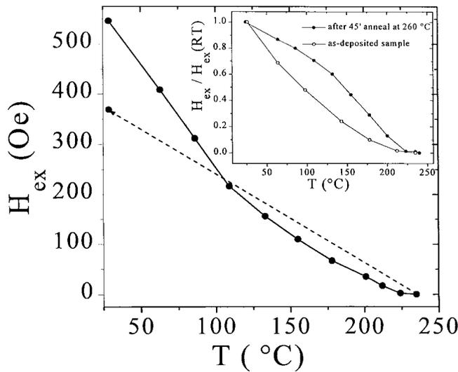
Fig. 4. Temperature dependence of the unidirectional exchange field  $H_{ex}$  for a Mn<sub>78</sub>Rh<sub>22</sub> biased spin valve coupon sample. The inset shows the effect of a 45 min anneal on  $H_{ex}(T)$ .
