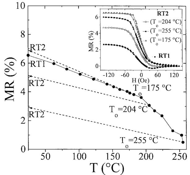
Fig. 5. MR signal versus temperature for unshielded spin valve sensors (trackwidth  $W = 6 \mu\text{m}$ , height  $h = 2 \mu\text{m}$ ). The dashed lines correspond to cycling back to room temperature, in the absence of an applied field. The inset shows the MR transfer curves for these sensors at RT after RT  $\rightarrow T_o \rightarrow$  RT.
