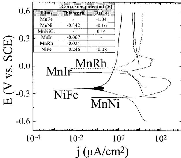
Fig. 3. Potentiodynamic polarized plots of as-deposited Mn<sub>78</sub>Rh<sub>22</sub>, Mn<sub>80</sub>Ir<sub>20</sub>, Ni<sub>81</sub>Fe<sub>19</sub>, and annealed Mn<sub>50</sub>Ni<sub>50</sub> films in a 0.1 N sodium sulfate electrolyte. Mn<sub>78</sub>Rh<sub>22</sub> shows a good corrosion behavior. In the inset, corrosion potentials of different materials measured at INESC are compared with previously published data.
