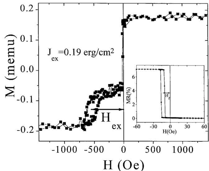
Fig. 2. Magnetization loop for a spin valve coupon sample with structure Si/Ta ( $50 \text{ \AA}$ )/ $\text{Ni}_{81}\text{Fe}_{19}$  ( $60 \text{ \AA}$ )/ $\text{Co}_{90}\text{Fe}_{10}$  ( $5 \text{ \AA}$ )/Cu ( $23 \text{ \AA}$ )/ $\text{Co}_{90}\text{Fe}_{10}$  ( $22 \text{ \AA}$ )/ $\text{Mn}_{78}\text{Rh}_{22}$  ( $170 \text{ \AA}$ )/Ta ( $50 \text{ \AA}$ ). The inset shows the minor MR loop.
